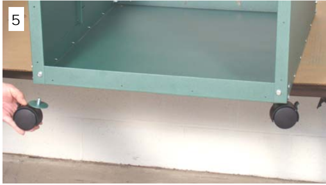
5) Install all (4) casters under the Bottom Panel, with a 1/2" flat washer and 1/2-13 nut on top. Tighten with a 3/4" wrench. OLD CASTERS SHOWN.
